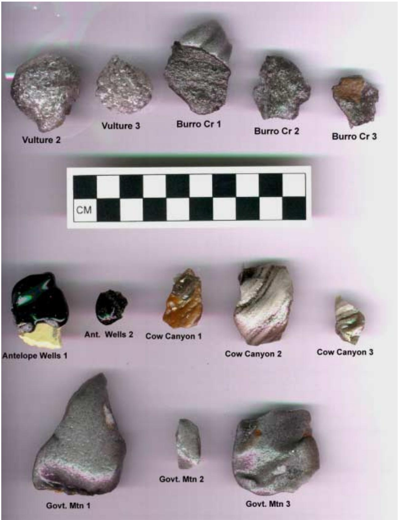
Figure 3. Samples after heating to 1080°C. Off-white material is the broken ceramic base plate incorporated into glass while heating to this temperature (see text).
